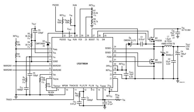
Figure 1. High Efficiency 5V-28V<sub>IN</sub> to 2.5V/10A Synchronous Buck Converter with Tracking and Margining
