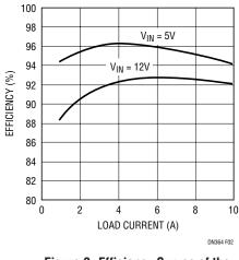
Figure 2. Efficiency Curves of the LTC3770 Converter in Figure 1
